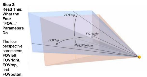
refer to the left, right, top and bottom sides of that display, as shown to the right. The frustum in pink shows the original, unmodified, view. Both views share a single view axis, which is the shortest perpendicular from the eye to the screen. In the unmodified view it is in the exact center of the screen. In the modified view, it is offcenter, because the frustum is deliberately lop-sided, as specified by the perspective parameters.
