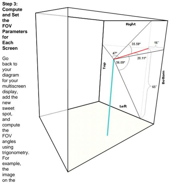
right shows a diagram of the BNAVE and the measurements for the right screen. The blue line roughly represents the viewer standing in the BNAVE, where the top of the line is the sweet spot. The Left/Right/Bottom/Top markings on the right side screen show what the game engine on that PC *thinks* is going on.
