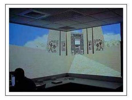
**BNAVE**, the three vertical walls are rear-projected and the one floor screen is front-projected from overhead.
