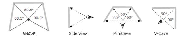
Three examples are shown on the right: the BNAVE (ignoring its floor), MiniCave, and V-Cave. The side view illustrates that the viewer's eye is level with the midpoint of each screen for each display.
