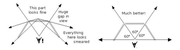
The drawing on the left shows a three-monitor flat display with the monitors turned inward.
