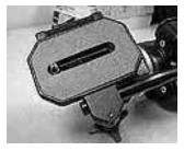
is mounted on the tripod, the tripod can rotate the projector a full 90 degrees to the right *and* a full 90 degrees to the left. This capability is needed for situations in which the projectors will need to be mounted sideways, so that the projection area can be taller than it is wide.
