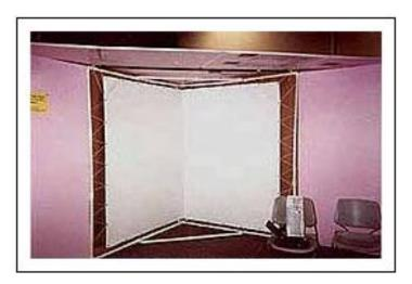
transparent and you are using front-projection, you must put something behind the screens to prevent light from leaking through the screens and washing out the projection image. Finally, there is single black bar supporting the frame's roof, which which is barely visible in the illustration to the right. This as just a water-pipe laid on top of the PVC pipe structure and tied onto the frame with two bits of rope.
