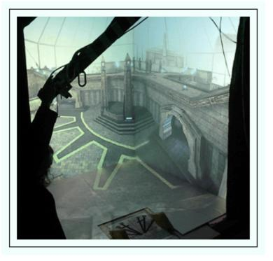
Each wall is a rear-projection screen. Onto each of the three screens is rear-projected projected the SVGA output of a dedicated PC.
