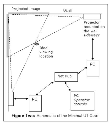
In this setup, two digital projectors are each mounted on a wall and pointed into the corner of a room, as shown in Figure One. Each projector displays on the wall perpendicular to its own. One edge of each projection lies along the corner itself, so the two images abut.
