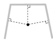
The diagram on the left shows where the sweet spot can be found for the BNAVE in an overhead view. Since all the screens are the same height, the vertical location of the sweet spot must be half the length of a screen up from the surface the BNAVE is resting on.
